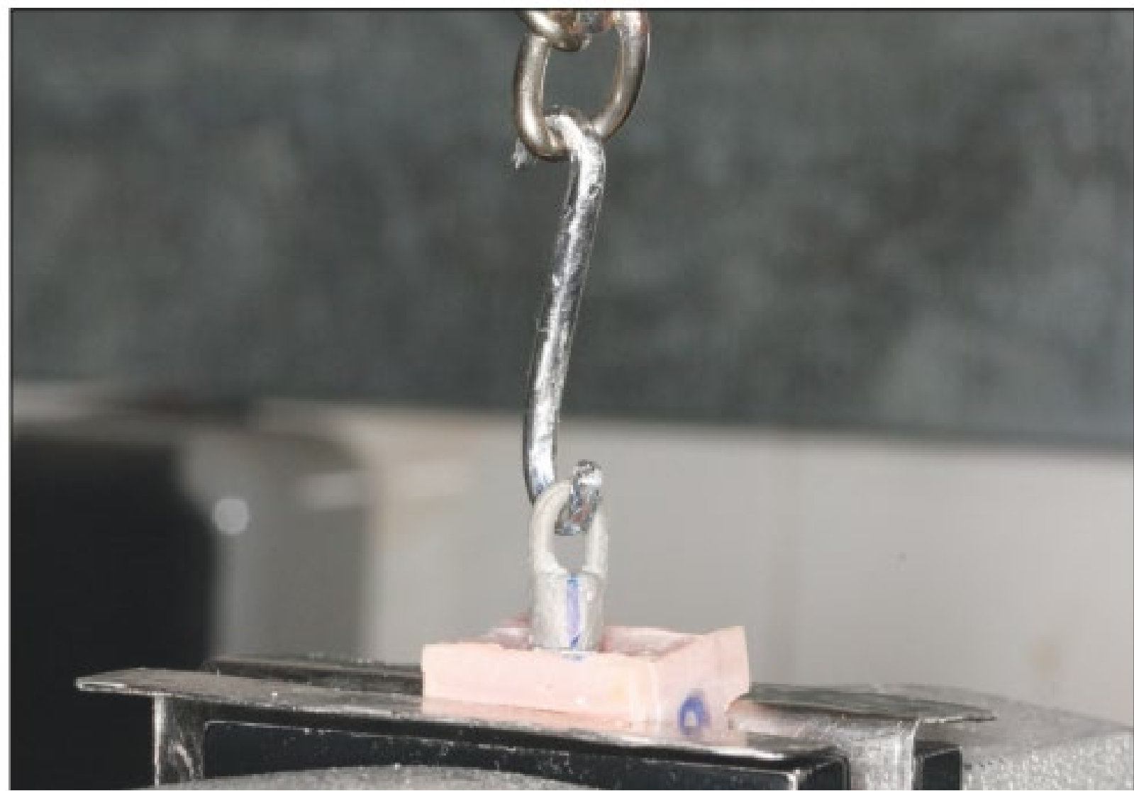
Luted metal coping during pull out test using universal testing machine 1
